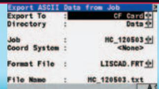
Data can be exported directly from TPS1200+ or via Leica Geo Office in various standard formats or in your own user-defined formats for direct input into any type of processing, office, CAD or mapping software.
