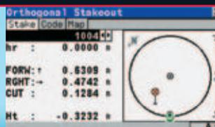
TPS1200+ is supplied with many useful programs such as Survey, Setup, Stakeout, COGO etc. Other programs such as RoadRunner, Reference line, Sets of Angles and DTM Stakeout are optional. You can also write your own programs for special applications in Geo C++.
