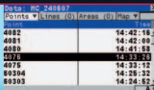
The powerful database manages data, files, jobs, quality checks etc. You can view, edit, delete, and search with or without filters. Coordinates of points measured more than once are averaged provided that they lie within specified tolerances.
