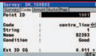
Define points, lines and areas to build up a plan in the display as you survey. You see immediately what you've done. Attach the codes, attributes and information needed for input into your office or mapping software.
