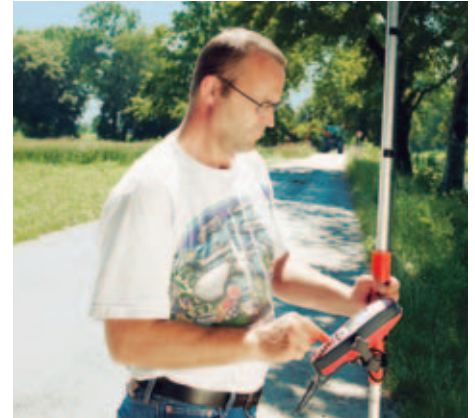
The SR20 being used to collect centimeter accurate topographic data using kinematic techniques.
