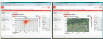
GeoMoS Web can graphically display time line, vector and scatter graphs. Data from multiple points and sensors can be used to help in the analysis.
